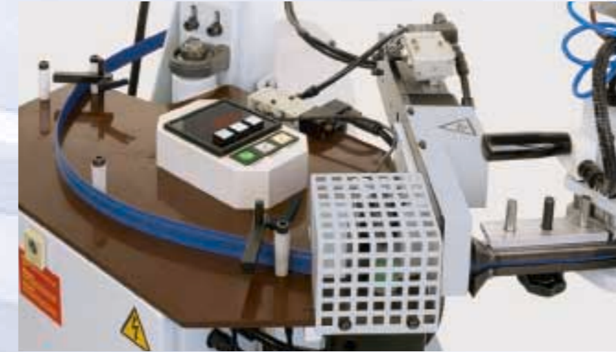
The edges are automatically cut to length according to input
