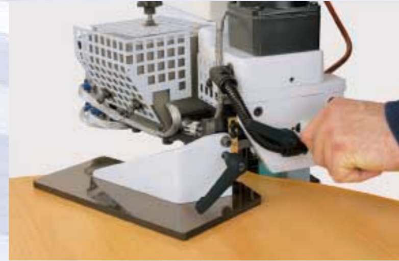
Guidance of the gluing unit by means of a height adjustable guiding plate
