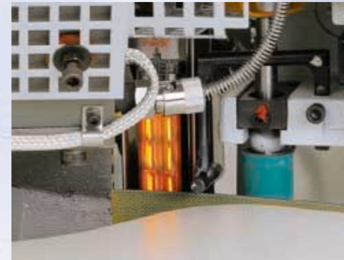
Infrared heating for thick PVC edgings
