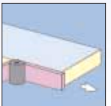
Processing of straight edges. Hot air unit for thick PVC edges (option).
